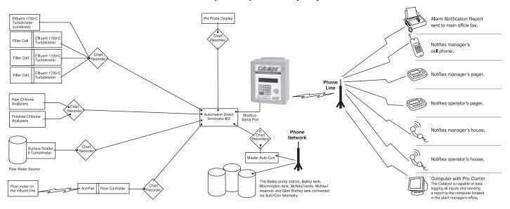
All units that require monitoring in Pike Township's system are connected to chart recorders, which send data to the Automation Direct Terminator I/O interface system. The interface system then sends the data to the Catalyst, which makes the appropriate alarm notification calls.
